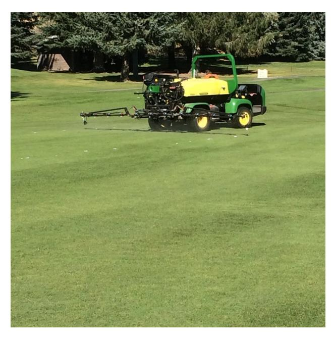
Figure 15. Foam markers help with spray accuracy.
