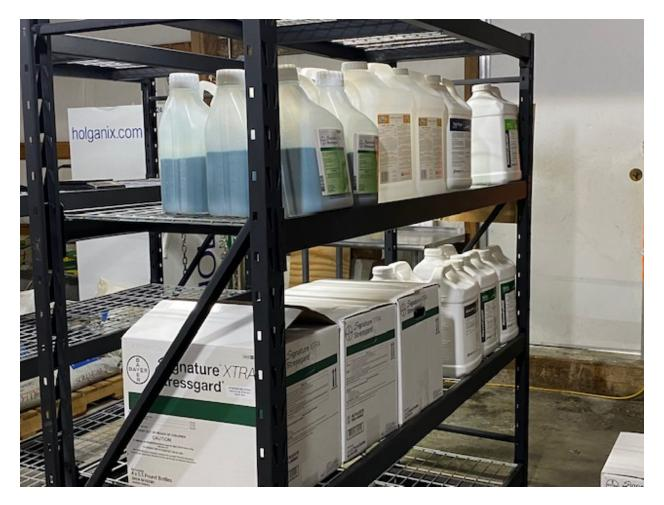
Figure 19. Wood shelving should never be used, because it may absorb spilled pesticides. Metal should be painted to stop corrosion. Photo credit: Kevin Glover.
