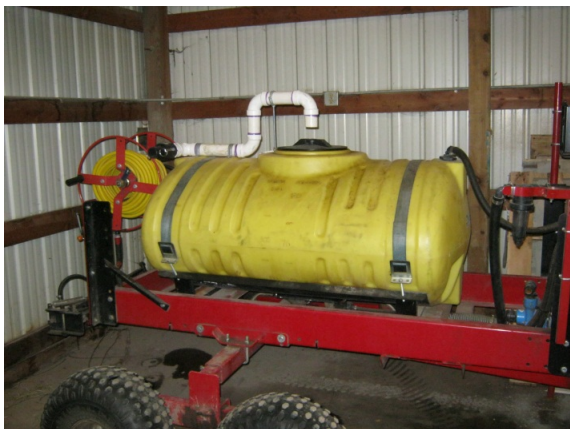
Fixed ridged air gap
