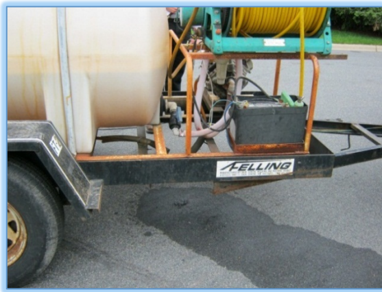
Leak from application equipment
