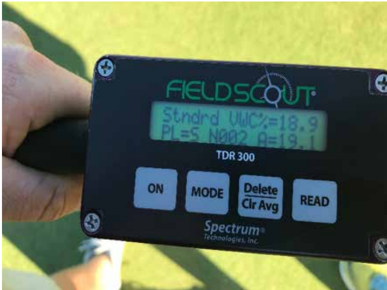
Digital reading of volumetric water content percentage and average moisture of green
