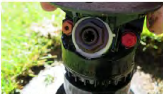
Sprinkler nozzles should be checked frequently for clogs and wear. Also, ensure that the proper nozzles are installed in each sprinkler.
