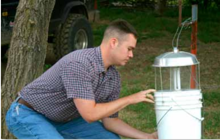
Light traps can be used as a scouting device to determine the presence and population levels of various insect pests, and thereby allow superintendents to initiate control measures in an accurate and timely fashion. Photo by Tom Royer
