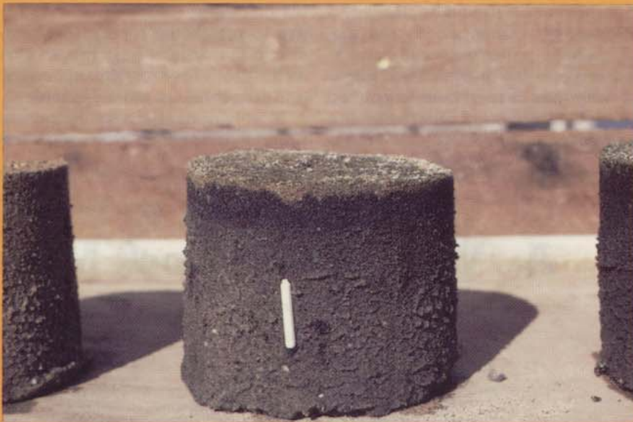
In contributing researchers' experiments, core samples (above) from experimentally produced black layers were all submerged in water for 33 days. The core designated "0" contained no added sulfur. Cores "1" and "5" received quantities of sulfur corresponding to 1 pound and 5 pounds of sulfur per 1,000 square feet. Where more sulfur was added, intensity of the layer increased. Note secondary growth of algae on cores "1" and "5"; algae growth is conspicuously absent on the core not receiving sulfur. Close-up photo (below) reflects the detailed appearance of the core receiving 1 pound of sulfur per 1,000 square feet.
