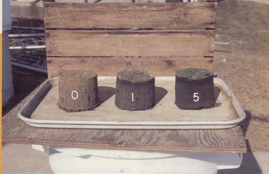
In contributing researchers' experiments, core samples (above) from experimentally produced black layers were all submerged in water for 33 days. The core designated "0" contained no added sulfur. Cores "1" and "5" received quantities of sulfur corresponding to 1 pound and 5 pounds of sulfur per 1,000 square feet. Where more sulfur was added, intensity of the layer increased. Note secondary growth of algae on cores "1" and "5"; algae growth is conspicuously absent on the core not receiving sulfur. Close-up photo (below) reflects the detailed appearance of the core receiving 1 pound of sulfur per 1,000 square feet.
