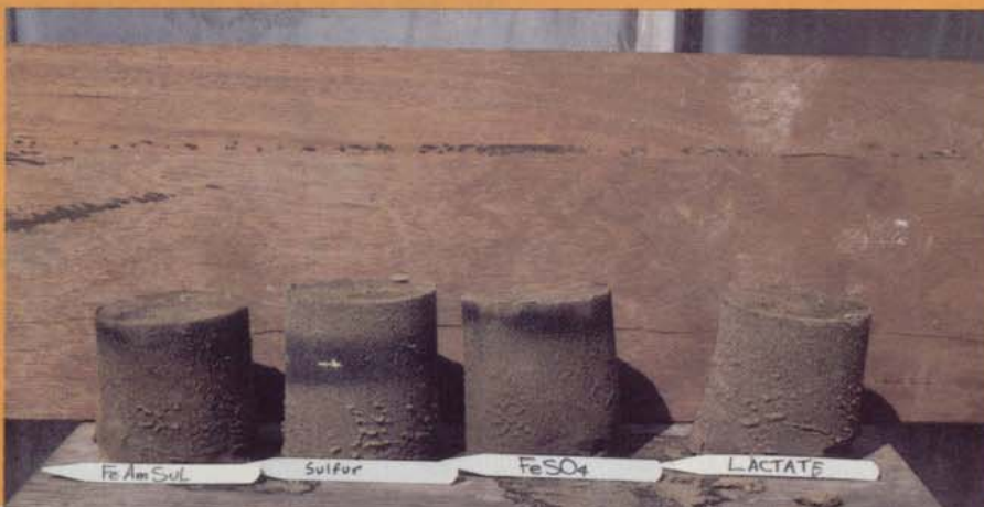
Other experimentally produced black layers (below) support a conclusion that compounds such as sulfur, ferrous sulfate ( \text{FeSO}_4 ) and ferrous ammonium sulfate ( \text{FeAmSul} ) will contribute to black layer formation.
