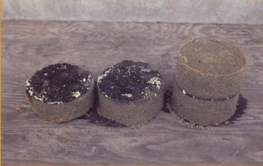
Pockets of remaining sulfur remain visible in this example of an experimentally produced black layer from a Lake Michigan sand dune. This layer was completely oxidized by atmospheric oxygen in less than 24 hours.
